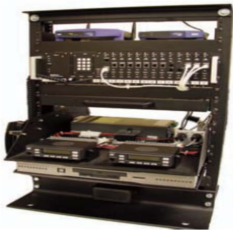
Photo caption: Left: A typical ACU1000 fixed site configuration. Top Right: ACU controller software. Bottom Right: WAIS controller software.
